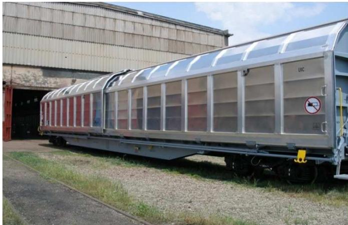
Railcar in operation with sliding walls in Hungary
